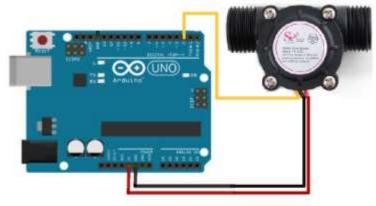
Figure 7.2 Connection of Arduino with Flow Sensor
